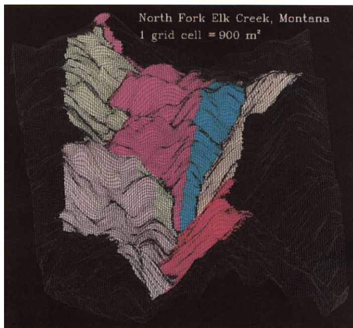
FIG. 6.5. Mesh diagram of a digital terrain model of North Fork Elk Creek, Montana, a 17 km 2 watershed used in ecosystem modeling experiments by NASA Ames researchers. Color draped over the mesh corresponds to the six hillslopes used to partition the area. Three IDL procedures were used to generate the picture: SURFACE, TRIANGULATE and POLYFILL.
