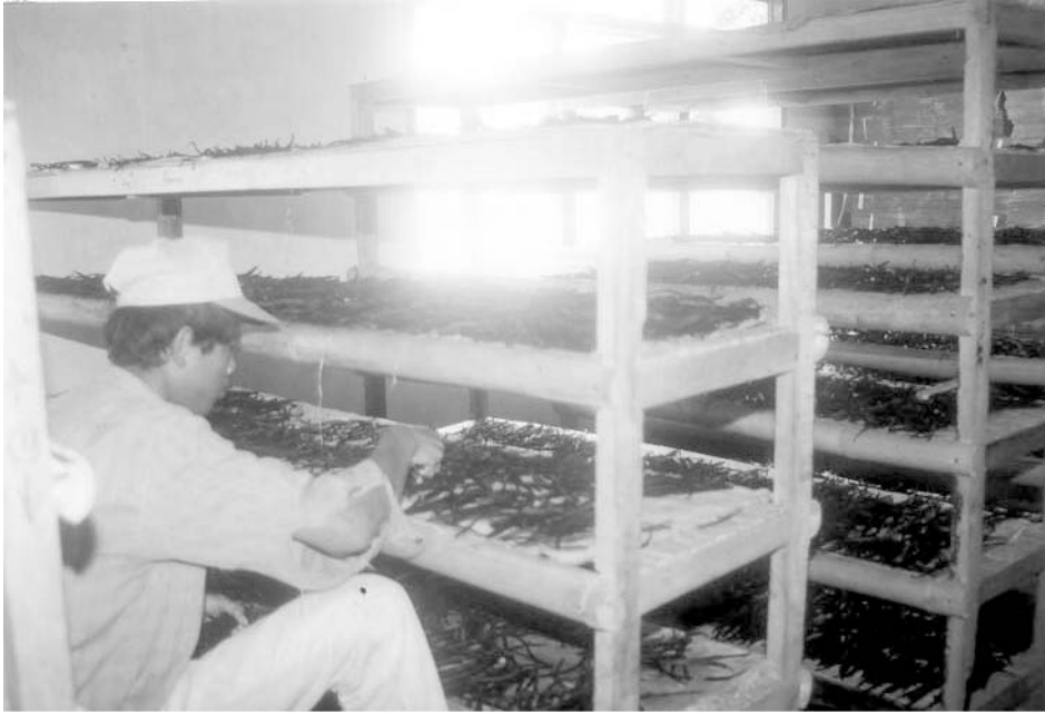
Fig. 20.7 Drying of cured beans in open shelves.
